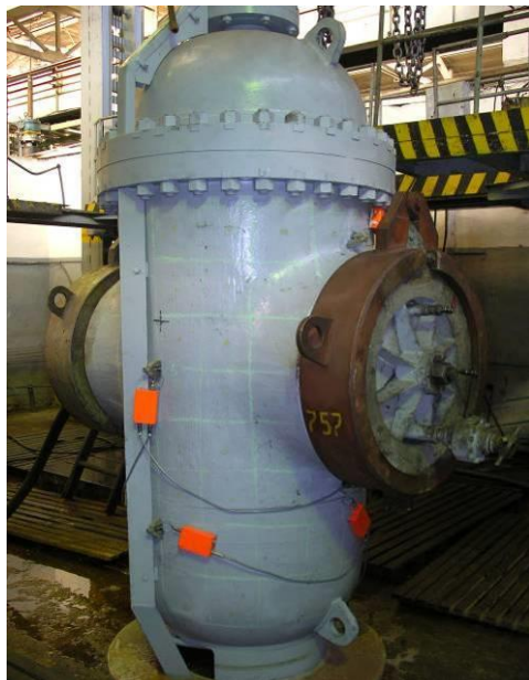
Gate valve under test
