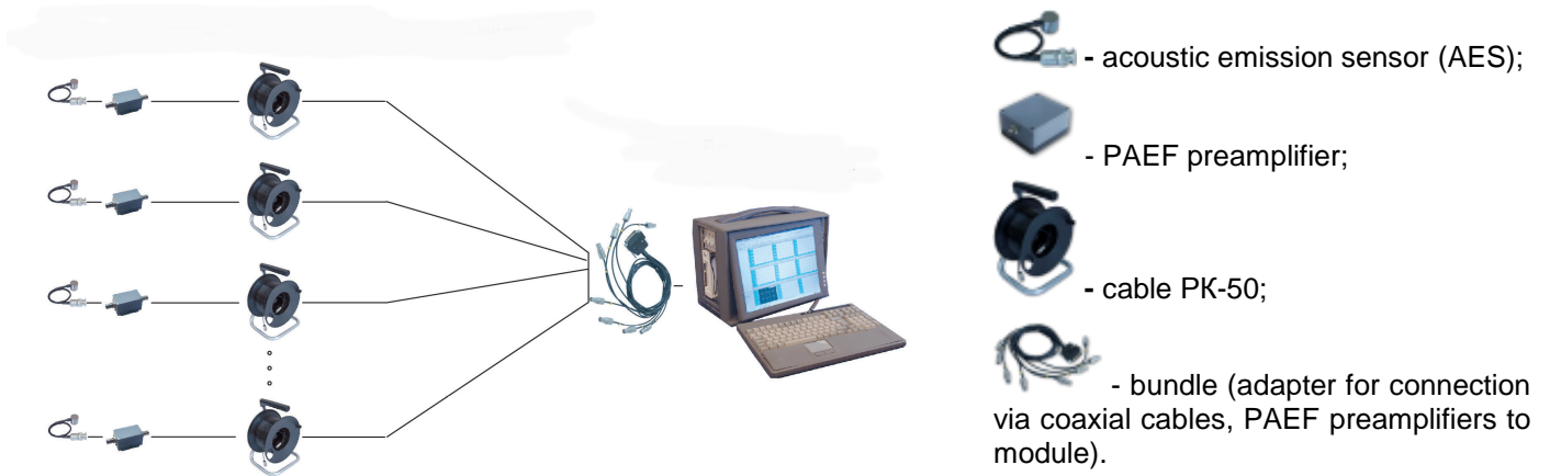
Structure scheme of A-Line 32D (PCI-8) AE system
